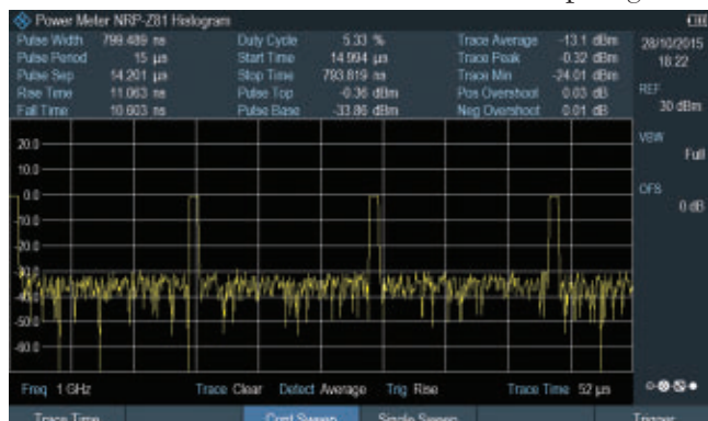
▲ Fig. 4 The R&S FPH-K29 option enables precise pulse and peak power measurements using the R&S NRP-Z8x wideband power sensor family.
